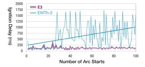
Testing has shown that ignition delay with E3 actually improves over time, while thoriated tungsten begins to deteriorate after only 25 starts.
