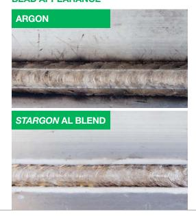
By increasing arc stability, arc energy and overall arc performance, Praxair's *Stargon* AL blend improves bead appearance, can reduce the cleaning zone, and provides better wetting and weld penetration – increasing process weld quality and operator appeal.
