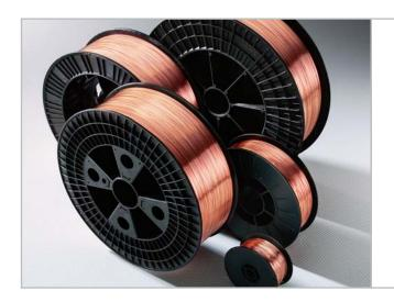
ProStar ER70S-6 wire is a mild steel welding wire with higher levels of deoxidizers (Mn and Si) compared to other mild steel welding wires. This wire is suitable for welding on mild steels with moderate amounts of scale or rust.
