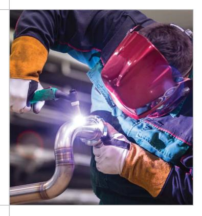
For stainless steel fabricators, *ProStar* stainless steel wire and electrodes are designed to provide good corrosion and crack-resistant welds with excellent welding characteristics and superior wetting.
