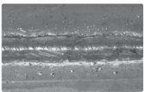
Chipping hammers clean the weld fillet
