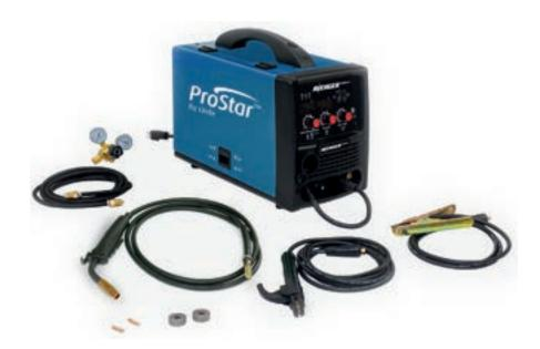
The PROSTAR<sup>TM</sup> AVENGER<sup>TM</sup> 140 MP MIG Welder is a portable, direct current (DC) inverter wire feed welder capable of welding with solid wire (with shielding gas) or with flux core wire. It comes ready to accept an optional spool gun for welding aluminum. This machine also has smooth DC stick capabilities and the ability to perform lift start DC gas tungsten arc (TIG) welding on steel and stainless steel materials with the optional TIG torch.
